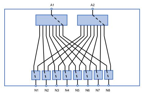
**Note:** the functional schematic is indicative of the switch matrix operation. Detailed wiring diagram can be found in the user manual
