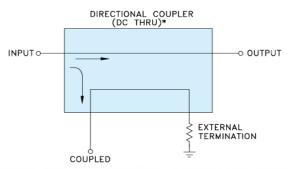
\* ELECTRICAL SCHEMATIC FOR DIRECTIONAL COUPLERS REQUIRING EXTERNAL TERMINATION THAT IS DESIGNED WITHOUT INTERNAL TRANSFORMERS.
