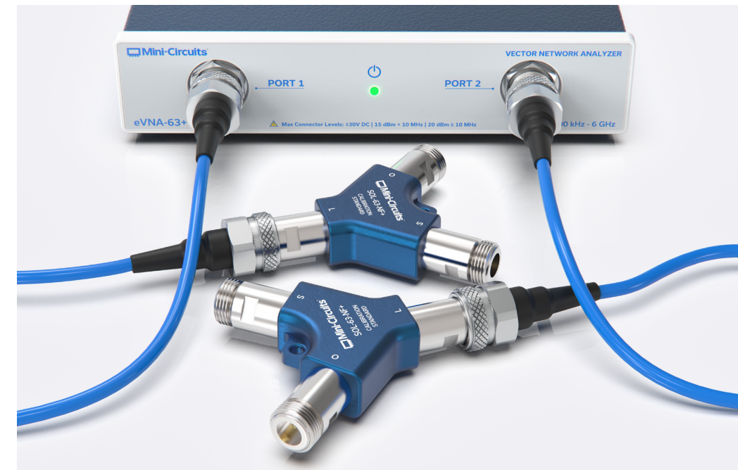
Figure 35: Load connections for response isolation calibration
