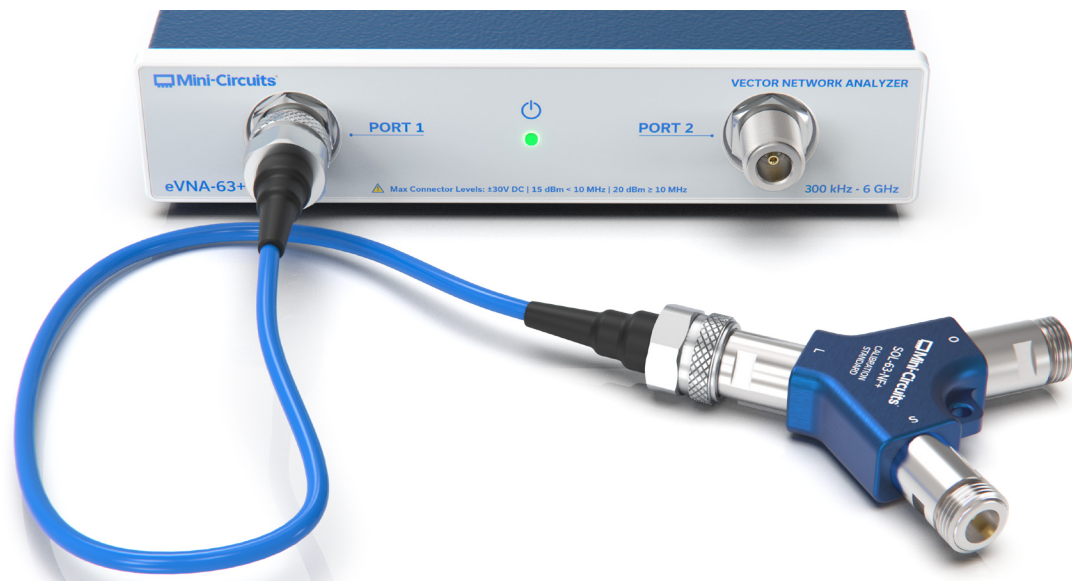
Figure 37: Load connection for response isolation calibration
