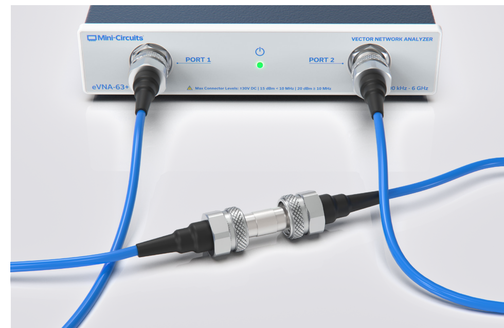
Figure 7: 2-port DUT connected with 2 sharply bent cables
