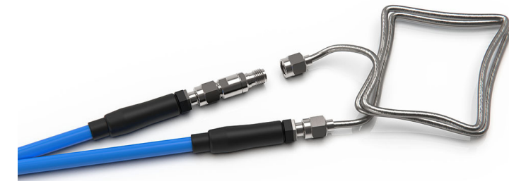
Figure 25: Male to female Thru connected on test cable 2—The same connector genders are now presented to the DUT
