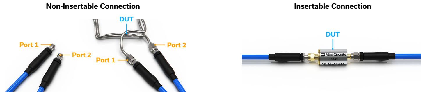
Figure 21: Examples of non-insertable (left) and insertable (right) devices
