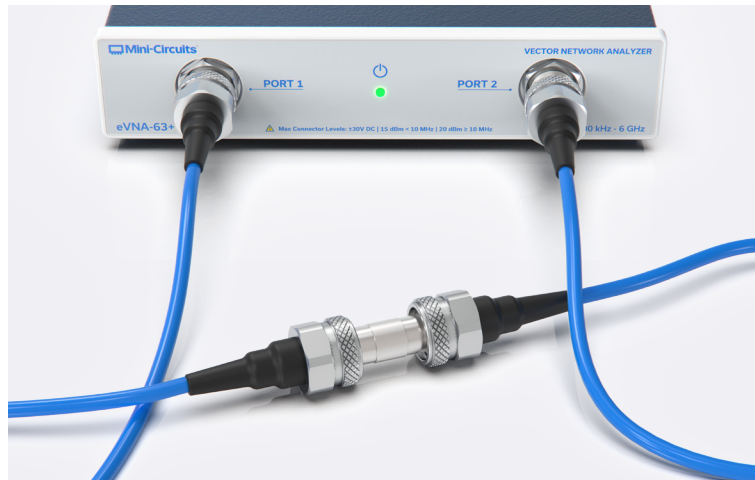
Figure 34: Thru connection for response thru calibration
