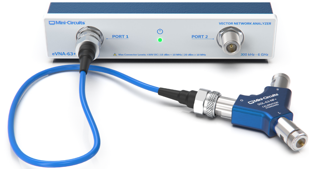
Figure 41: Measurement setup for 1-port calibration
