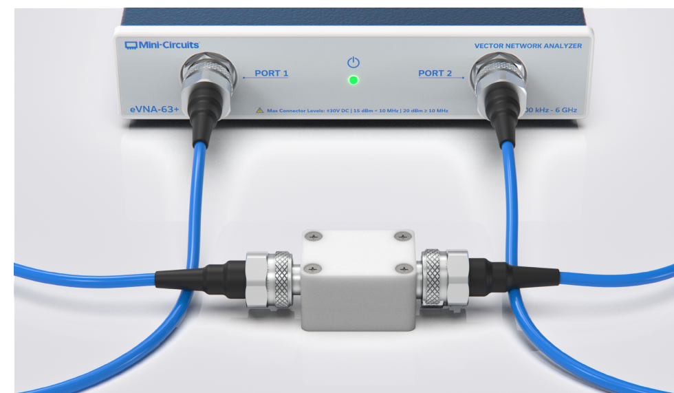
Figure 8: 2-port DUT connected with 2 longer cables to allow gentle bend
