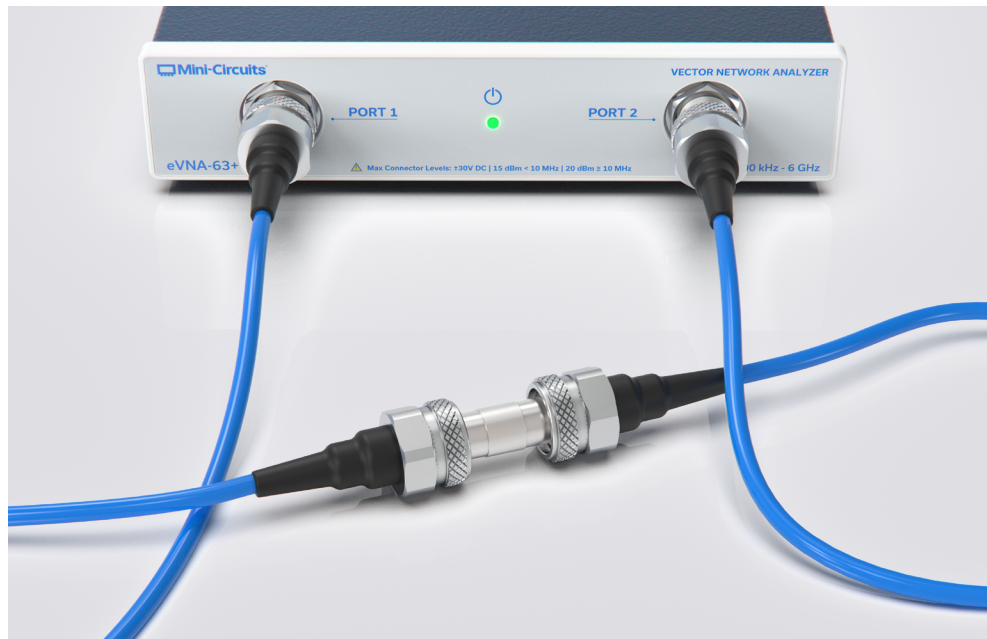
Figure 39: Thru connection for enhanced response calibration
