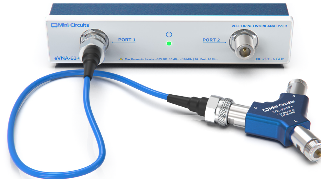
Figure 36: Open connection for response reflection calibration
