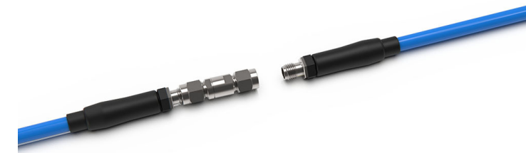
Figure 24: Male to male Thru, used to interconnect the two VNA test cables
