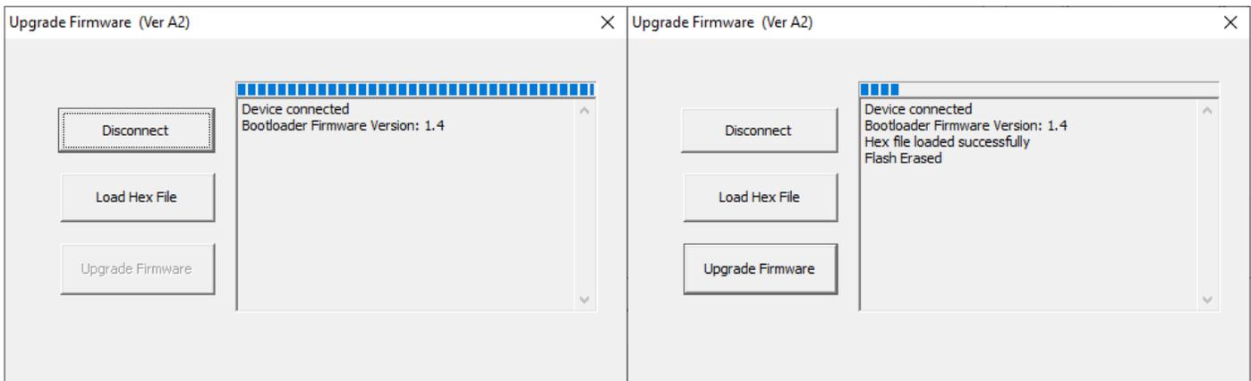
**Figure 3.9.2** Firmware Upgrade App. (Connection step – left, Upgrade step – right)
