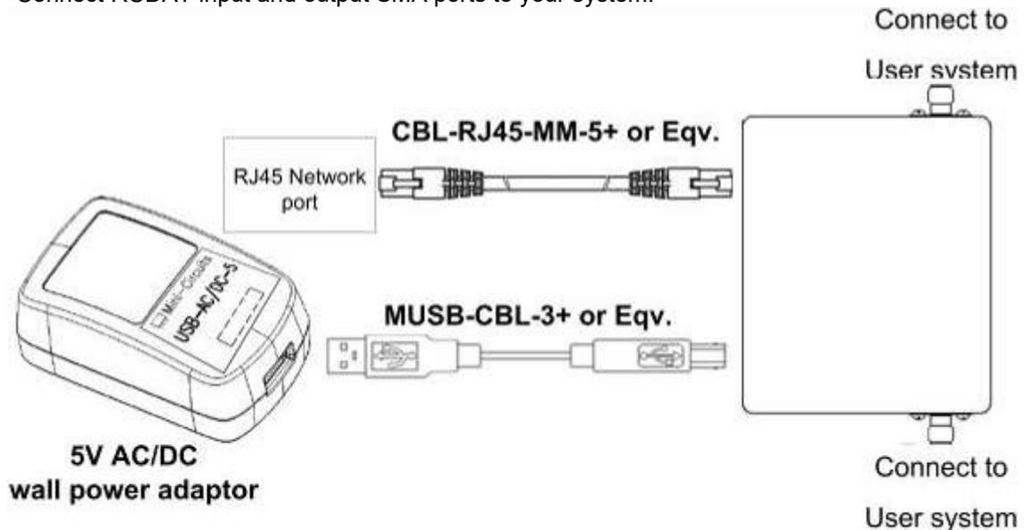
Figure 2.3.4: RCDAT Ethernet setup
