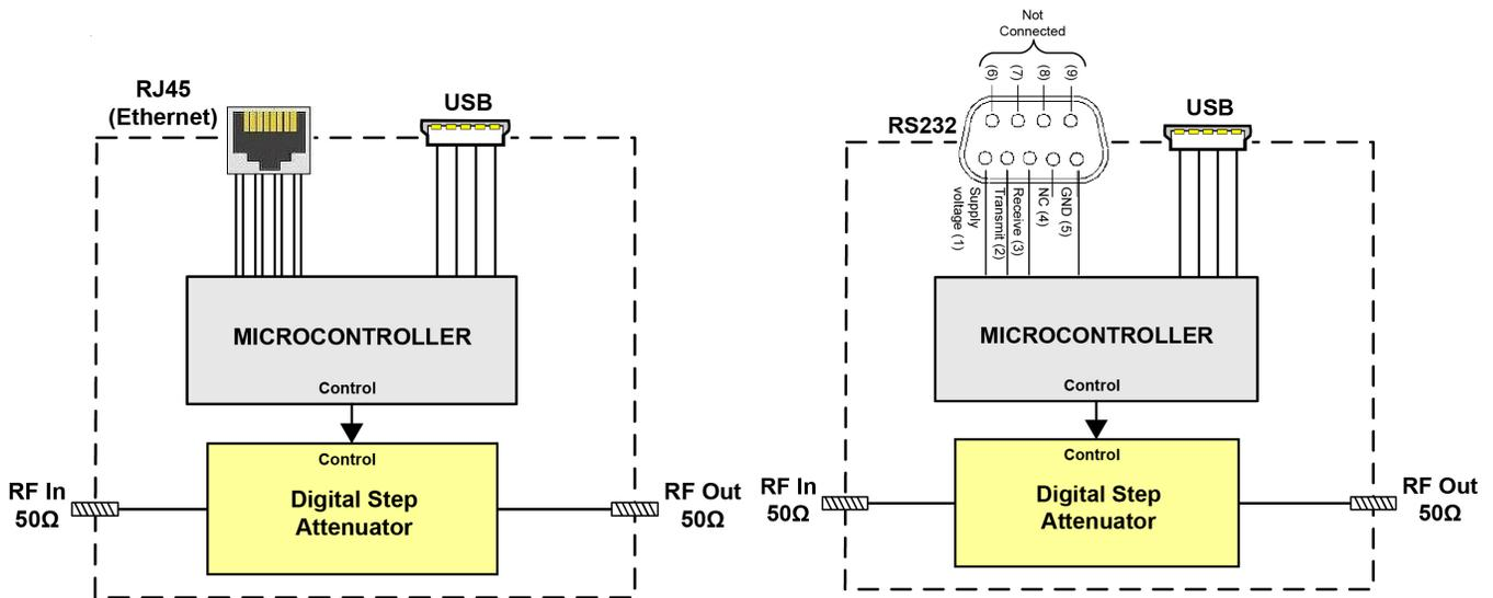
Figure 1.8.2a RUDAT & RCDAT functional block diagrams
