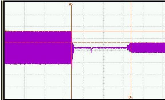
**Figure 3.5.3c:** Typ. Switching time from 10 to 0 dB(RUDAT-13G-90); 600 ns switching time
