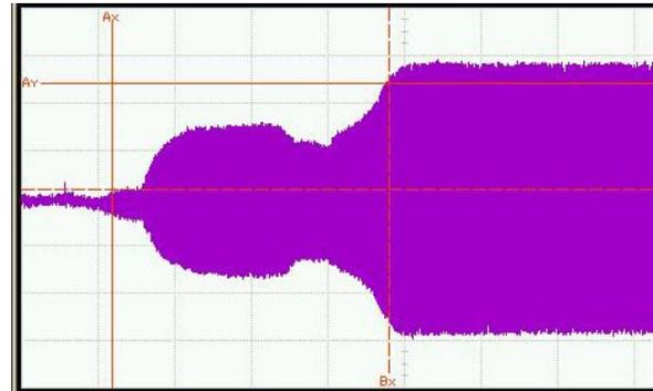
**Figure 3.5.3b:** Typ. Switching time from 45 to 15 dB(RCDAT-4000-120); 362 ns switching
