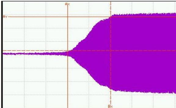
**Figure 3.5.3a:** Typ. Switching time from 120 to 0 dB(RCDAT-4000-120); 200 ns switching time
