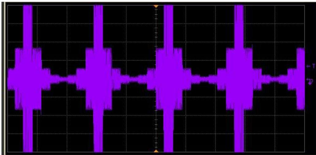
**Figure 3.5:** Plot of signal when sweeping attenuation 0-40dB in 10 dB steps (scale 2ms/div)
