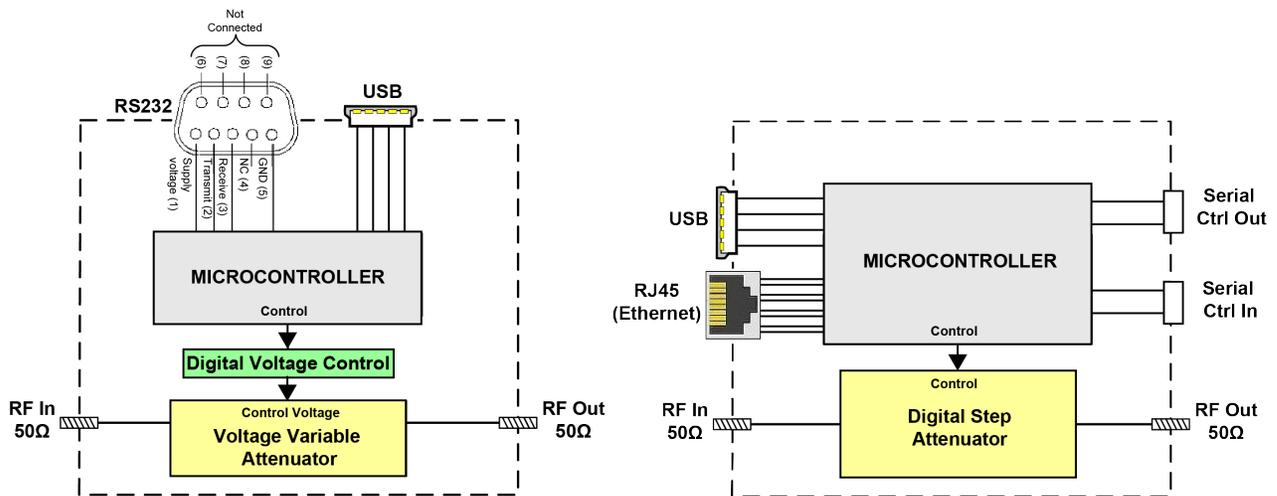
Figure 1.8.2b ZVVA & RCDAT with dynamic addressing functional block diagram
