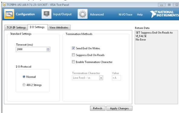
Fig xii - Uncheck the "Supress End on Reads" option
