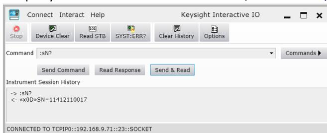
Fig x - Requesting the serial number; the response is 11412110017
