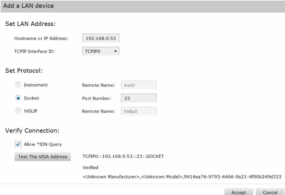
Fig ii - The successfully tested LAN device settings for a power sensor with IP address 192.168.9.53
