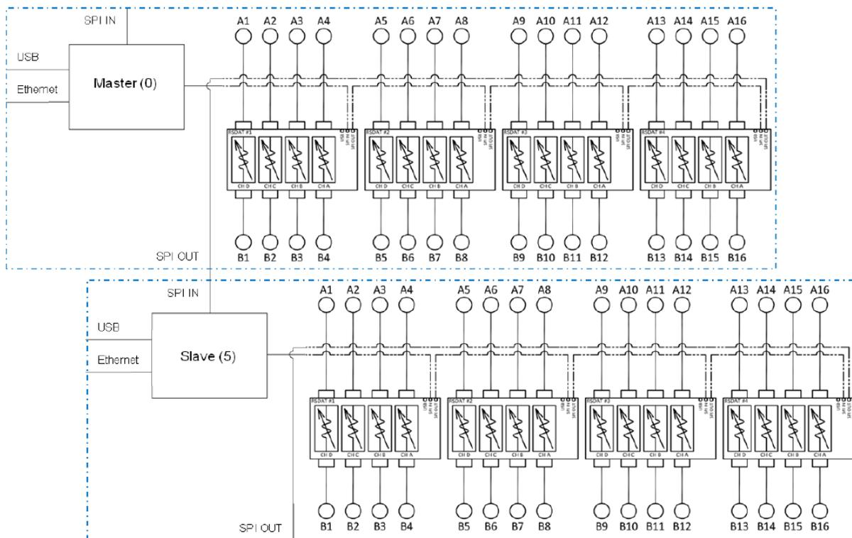
Figure 1: Block Diagram of 2 ZTDAT-16-6G95S Daisy Chained Together
