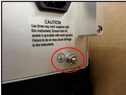
Figure 8: Rear panel grounding terminal
