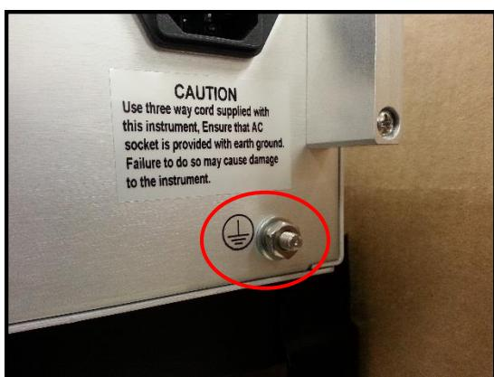
Figure 8: Rear panel grounding terminal
