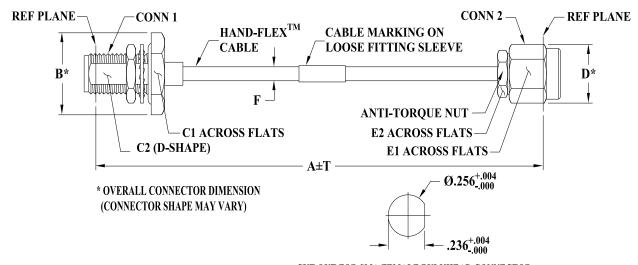
CUT OUT FOR SMA FEMALE BULKHEAD CONNECTOR PANEL THICKNESS .100 MAX INCHES
