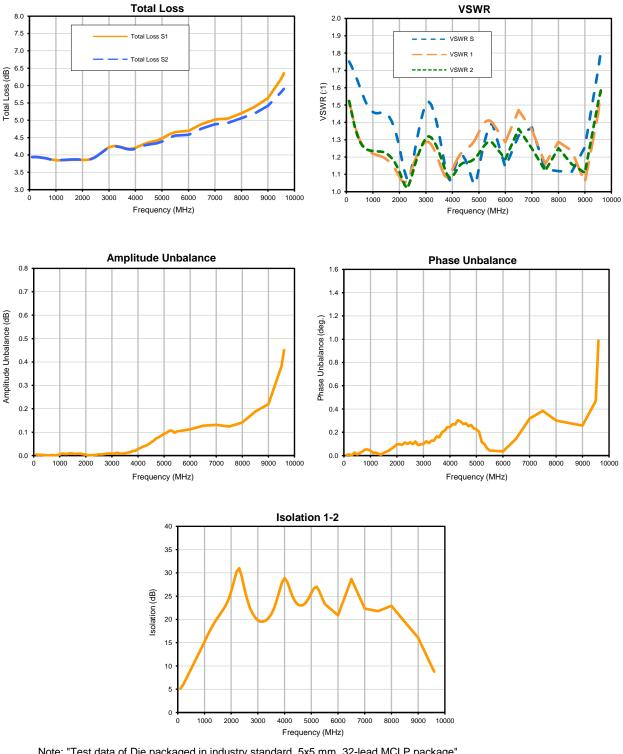
Note: "Test data of Die packaged in industry standard, 5x5 mm, 32-lead MCLP package"
