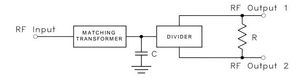
Figure 1 shows a block diagram of a power splitter. It consists of an input matching section, a divider section, a capacitor and a resistor. In a 50-ohm system, the impedance at the input of the divider is close to 25 ohms. The matching transformer converts this to 50 ohms at the RF input to provide a good match. Normally a capacitor C is required to match the reactive part of the impedance. The resistor R plays a critical role in providing isolation between the two RF out put ports.
