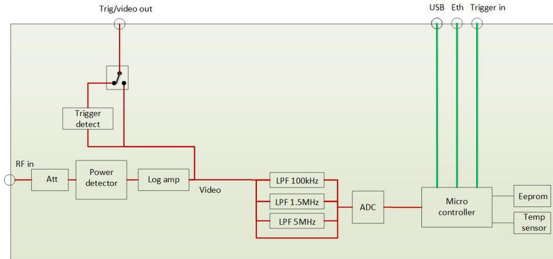
*PWR-40PW-RC functional block diagram*
