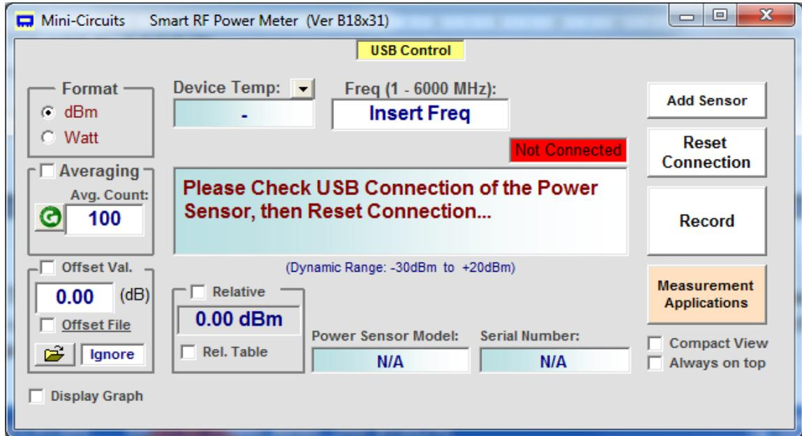
If there's a faulty DUT connection, no RF power or the power is below the sensors dynamic range a 'Power Too Low' notice will appear.
