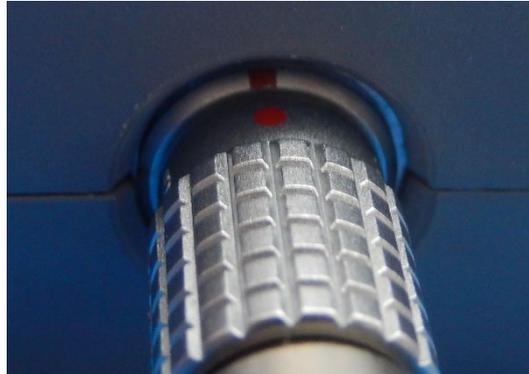
Figure 4.1: Plug cable into unit.
