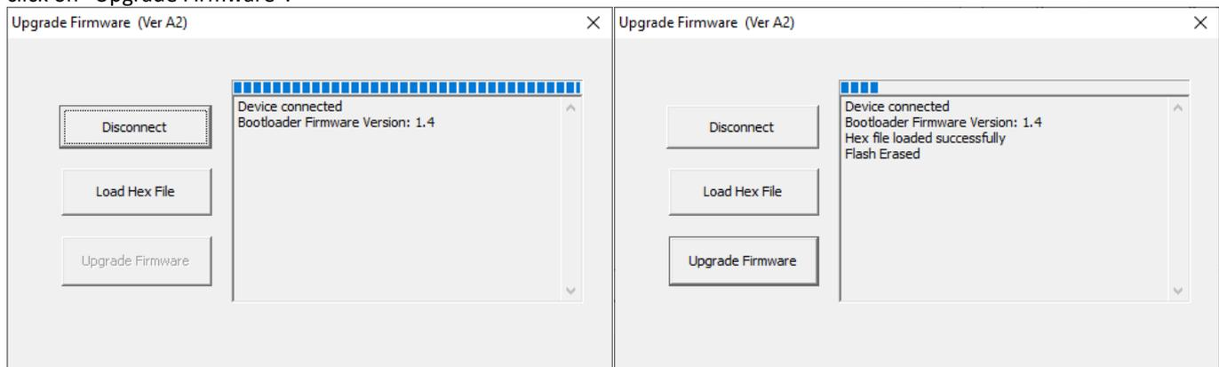
*Firmware Upgrade App for PWR-40PW-RC & PWR-8PW-RC. (Connection step – left, Upgrade step – right)*
