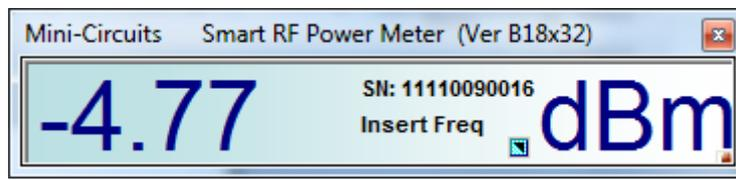
Clicking on any spot in the 'Compact View' screen will cause the program to return to the main screen. In compact view the program displays power measurement, measurement units, Power sensor S/N, and the frequency entered but you must return to main screen to change any parameters.
