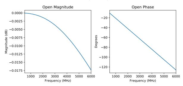
Figure 3: Model for the 85033D/E Cal. Kit Open Standard, Magnitude (left), Phase (right)
