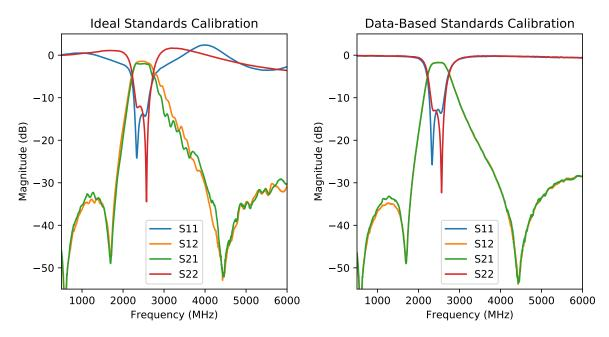
Figure 1: UVNA-63 kit measurement of a 2.5 GHz bandpass filter with ideal SOLT calibration (left) and data-based SOLT calibration (right)
