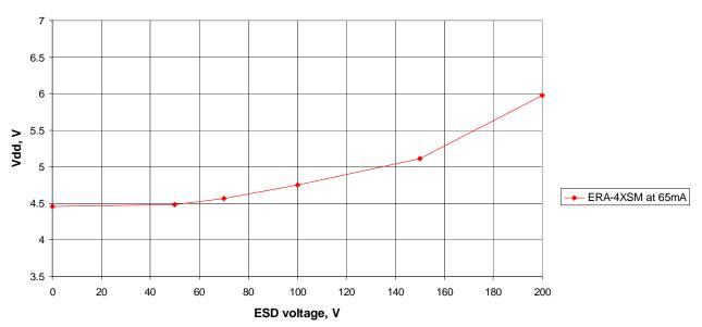
Figures 1 and 2 show that very little but still noticeable degradation in gain (0.1dB) and device voltage (0.1V) starts with the 70V ESD pulse.
