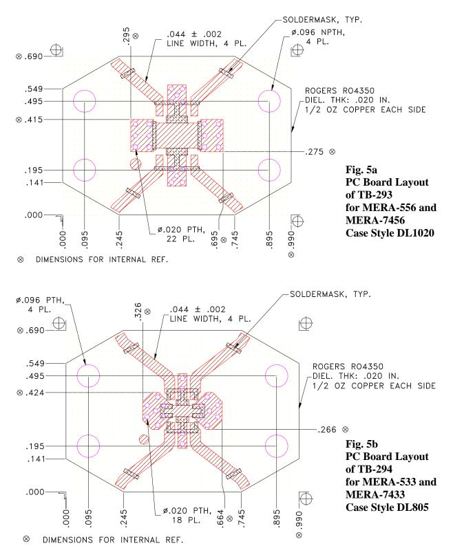
Figure 5 – PC Board Layouts used in Mini-Circuits Test Boards
