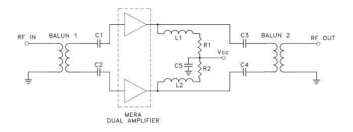
Figure 6 – Push-Pull Amplifier using MERA
