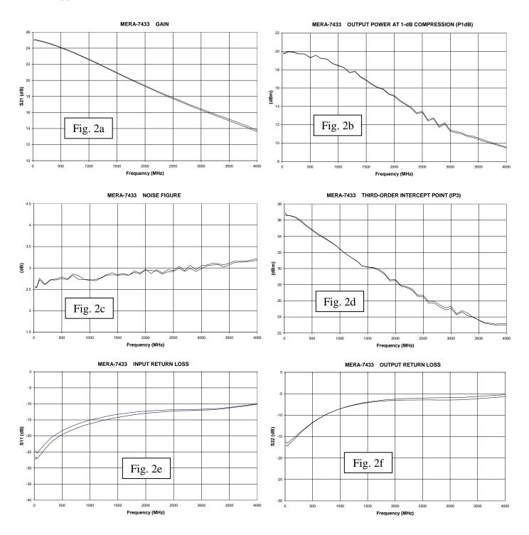
Figure 2 – Typical Performance of Dual Amplifier MERA-7433 at 25°C
