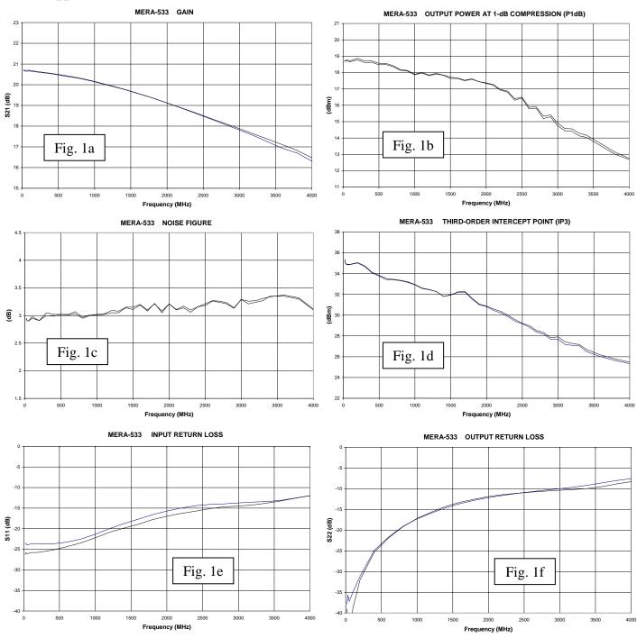
Figure 1 – Typical Performance of Dual Amplifier MERA-533 at 25°C
