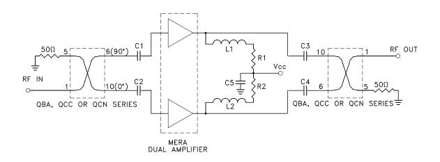
Figure 7 – Balanced Amplifier using MERA
