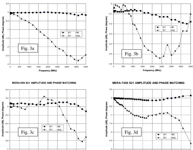
Figure 3 – Typical Gain Matching of the 4 Models at 25°C: Amplitude and Phase
