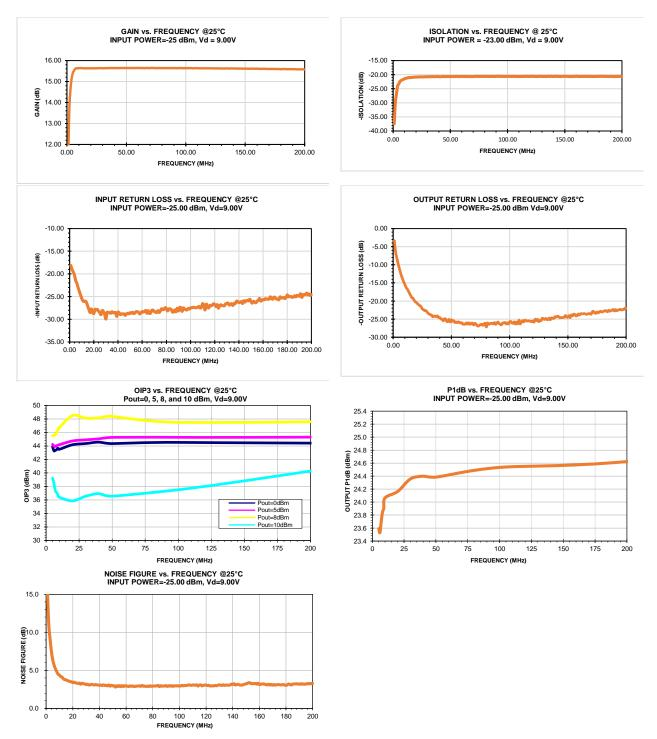
Figure 5: Plots of measured performance of PGA-122-75+ in alternative application circuit swept over 5 to 200 MHz.
