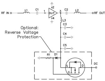
Component Value Size DUT PGA-122-75+ -C1 1000 pF C2 120 pF 0402 100 pF C3 C4 10000 pF C5 10 µF, 25V 1206 Zener Diode 5.6V D1 ONSEMI **SOD123** MMSZ4690T1G L1 3.3 nH 0402 L2 4.7 nH L3 560 nH 0603 R1 1.5 kOhm Transistor Q1 **ONSEMI FET** SOT323 NTS4101P
