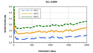
Figure 2: Plots of measured performance of PGA-122-75+ in recommended application circuit (downstream).
