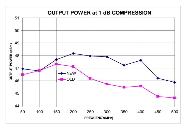
Graph 6 OUTPUT POWER at 1 dB COMPRESSION vs FREQUENCY
