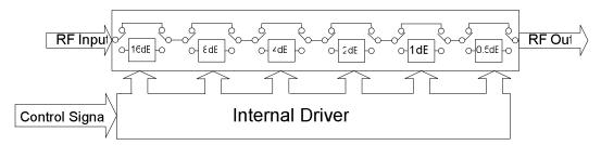
Fig. 1: Simplified schematic of a 6 bit digital attenuator.
