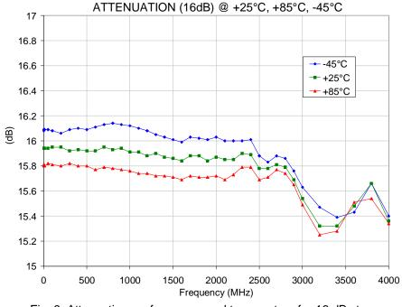
Fig. 3: Attenuation vs. frequency and temperature for 16 dB step
