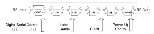
Fig. 10: Functional schematic of a 6 bit attenuator with serial control.
