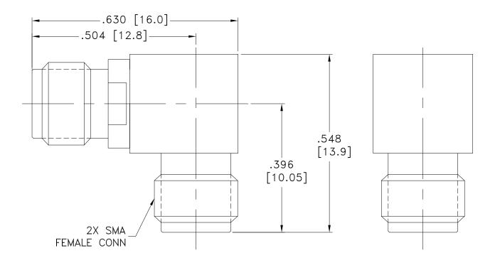
Weight: 6.5 gram Dimensions are in inches (mm). Tolerances: 2 Pl. <u>+</u> .030; 3Pl. + .015
