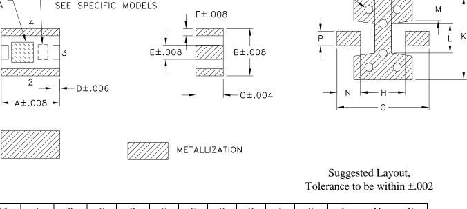
Q TYP PLATED THRU HOLE ON GROUND PAD
