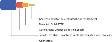
Coupling Nut: Stainless Steel Passivated Body: Stainless Steel Gold Plated Center Pin: Silver Plated Copper Clad Steel
