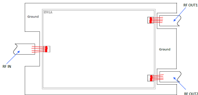
Four 1 mil bond wires should be used for RF input and RF output.
