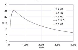
S22 (-Output Return Loss) vs. Frequency & Rb
