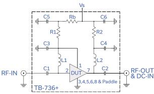
Fig 1. Application and Characterization Circuit Note: This block diagram is used for characterization. (DUT soldered on Mini-Circuits Characterization test board TB-736+)
