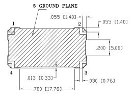
NDTES: 1. DIMENSIONS INCH [MM]. 2. PIN NUMBERS DO NOT APPEAR ON UNIT, FOR REFERENCE ONLY. METALLIZATION SOLDER RESIST
