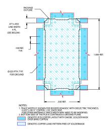
Figure 2. Suggested PCB Layout PL-469
