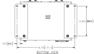
SHOWN WITH RUBBER FEET REMOVED AND BRACKETS INSTALLED
