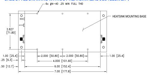
Weight: 900.0 grams. Weight without heatsink: 600.0 grams Dimensions are in inches [mm]. Tolerances: 2 Pl.±03; 3 Pl. ±.015 Inch
